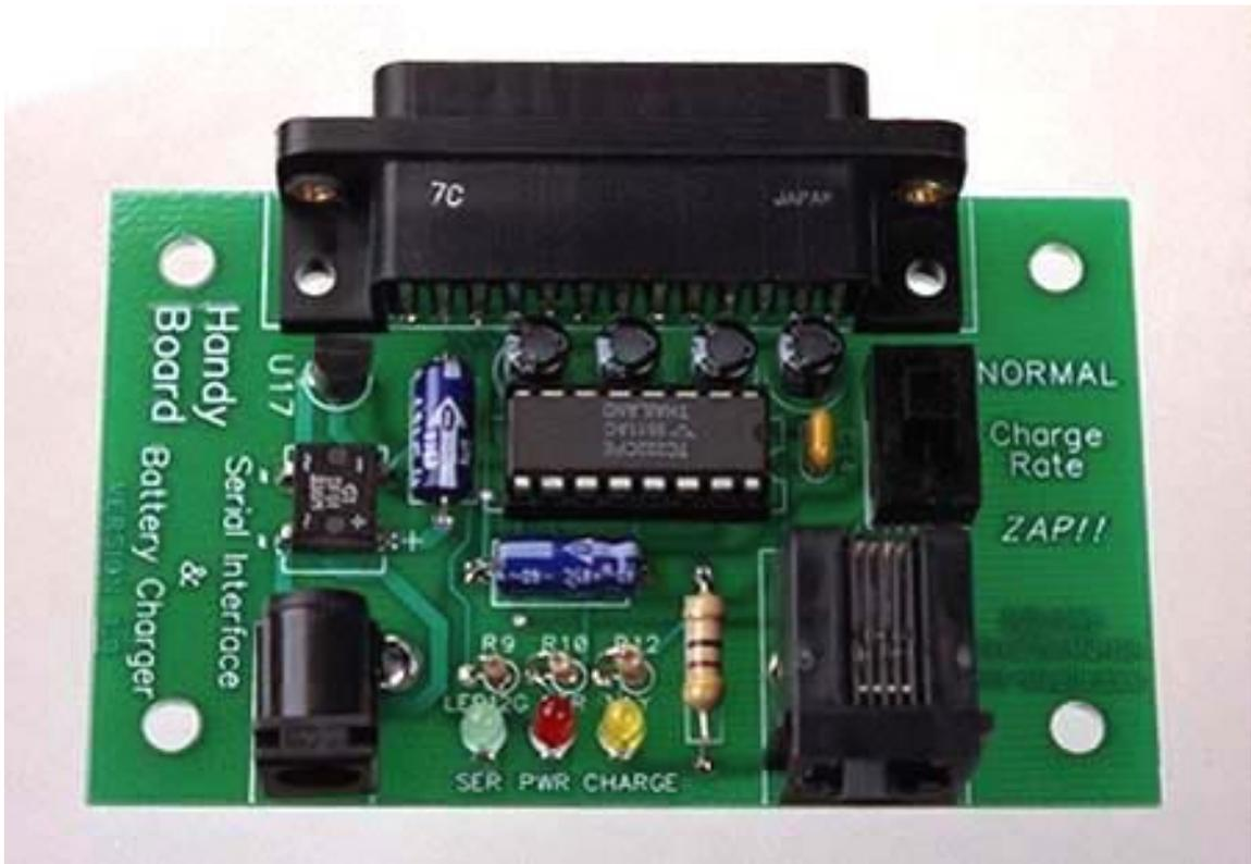
Figure 5: Interface/Charger Board, Charge Circuit and Jacks
