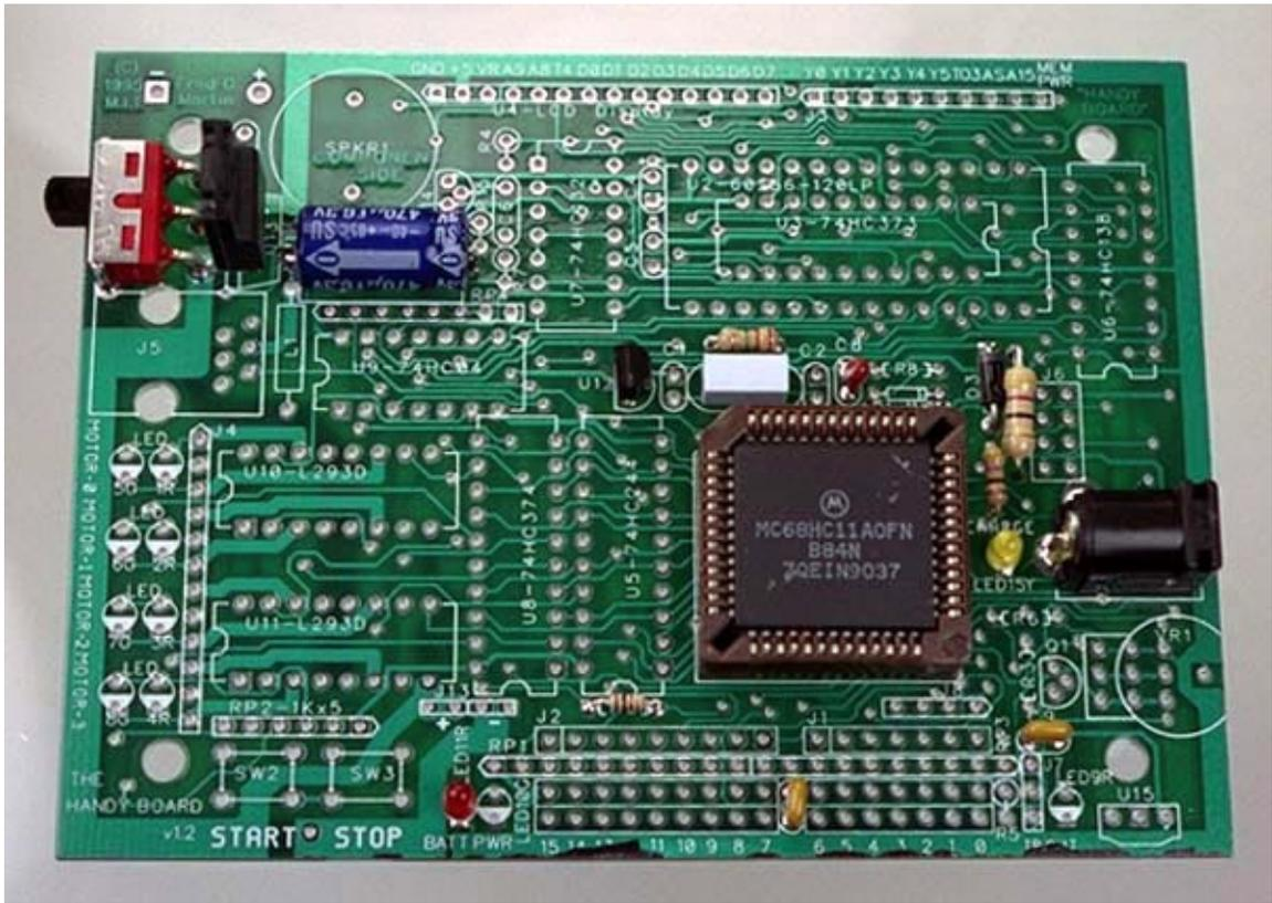
Figure 8: Microprocessor and Oscillator Circuit
