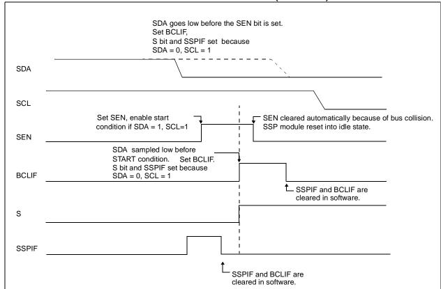
FIGURE 9-21: BUS COLLISION DURING START CONDITION (SCL = 0)
