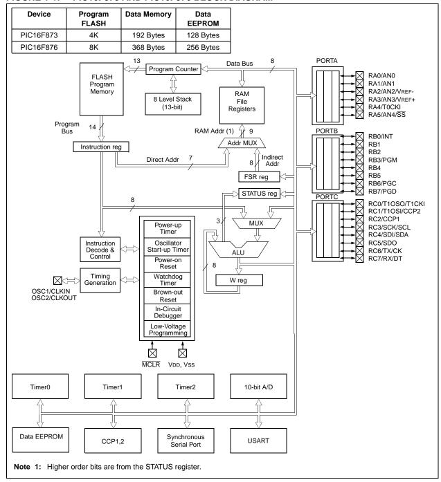
FIGURE 1-2: PIC16F874 AND PIC16F877 BLOCK DIAGRAM
