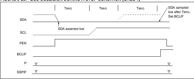
FIGURE 9-26: BUS COLLISION DURING A STOP CONDITION (CASE 2)
