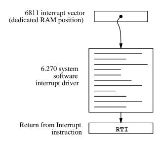
Interrupt-driven binary programs use the initialization sequence of the binary module to install a piece of code into the interrupt structure of the 6811.
