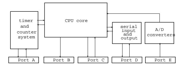
Figure 6: Simplified Block Diagram of 6811
