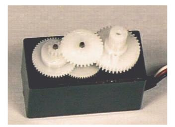
• Be careful to note how the gears are arranged, and remove them from the top of the servo. I usually place them as the are supposed to sit. The large fine tooth gear in the middle does not need to be removed. See the picture below.
