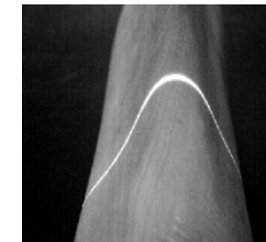
Detail of the polyline generated by the laser plane.
