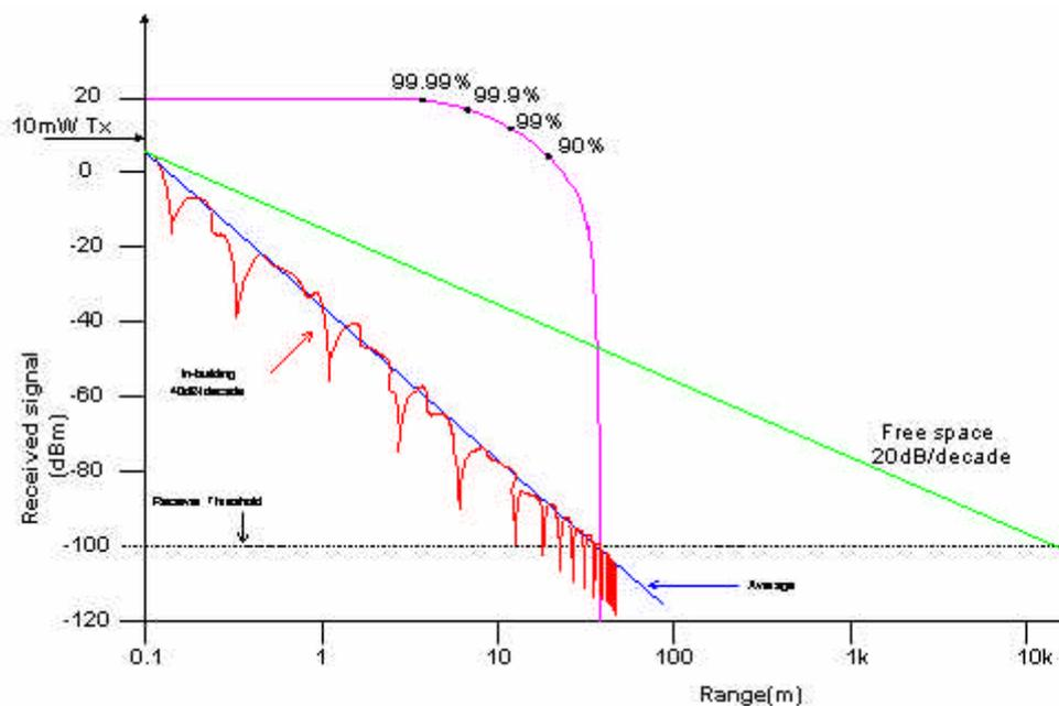
*curve for a 433MHz 10mW TX (unity gain antenna)*
