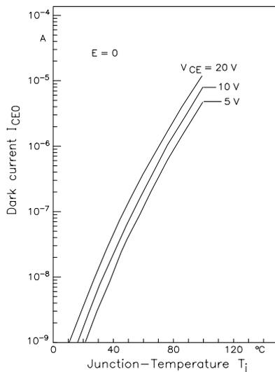
Figure 10. Temperature-dependence of the collector dark current
