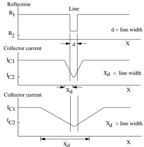
Figure 8. Reflection of a line of width  $d$  and corresponding curve of the collector current  $I_c$
