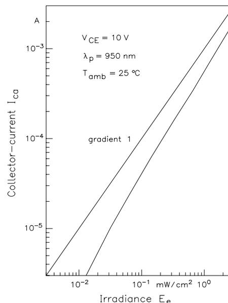
Figure 2. Sensitivity of the reflex sensors' detector
