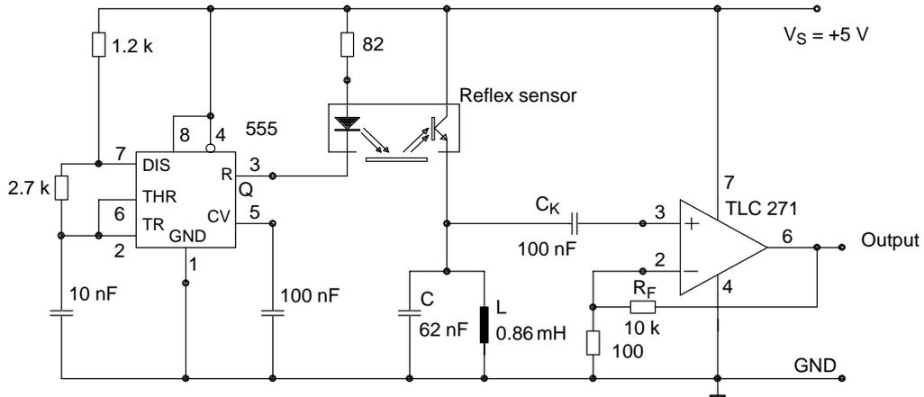
Figure 14. AC operation with oscillating circuit to suppress ambient light
