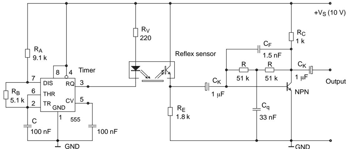
Timer dimensions:  $t_p$  (pulse width) =  $0.8 RC = 400$  ms
