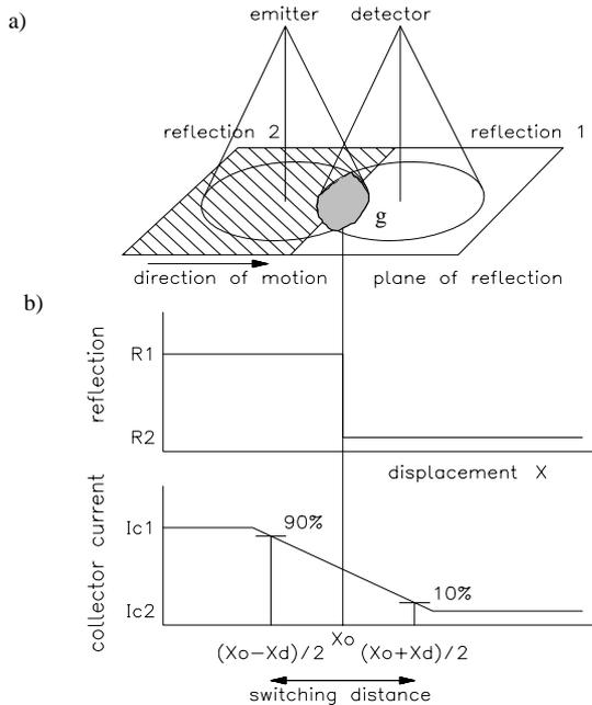
Figure 7. Abrupt reflection change with associated  $I_c$  curve
