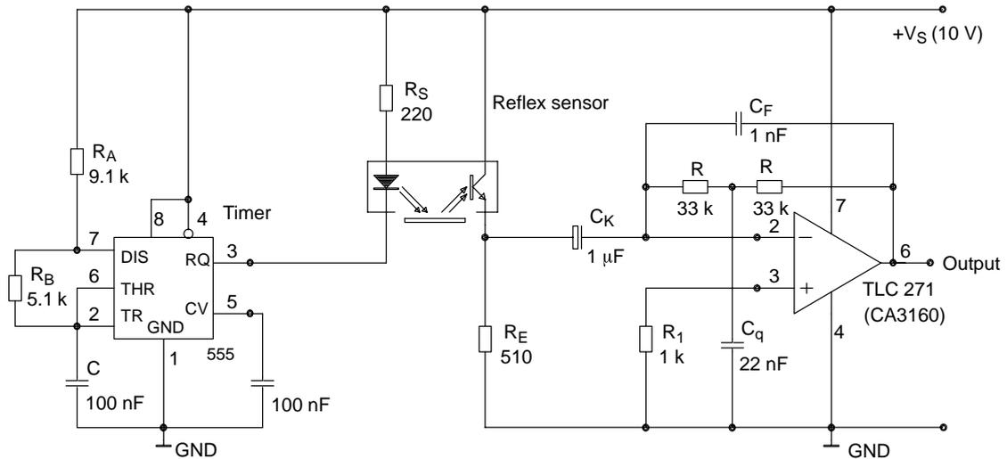
Timer dimensions:  $t_p$  (pulse width) =  $0.8 RC = 400 \mu s$
