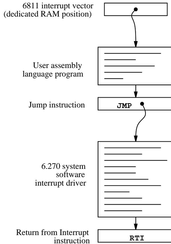
The first figure depicts the interrupt structure before user program installation. The 6811 vector location points to system software code, which terminates in a “return from interrupt” instruction.
