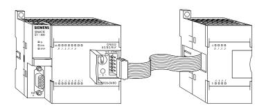
The ribbon connector is protected by a cover on the base unit. Side-by-side mounting completely encloses and protects the ribbon connector.
