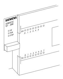
The I/O status indicators represent the On or Off status of corresponding inputs and outputs. When the CPU senses an input is on, the corresponding green indicator is lit.
