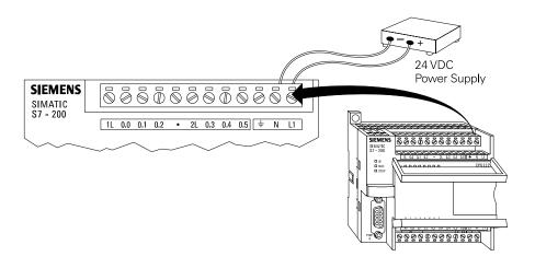
An S7-200 AC/DC/Relay would be connected to a 120 or 230 VAC power supply.
