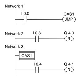
If 10.0 = "1", the jump to label CAS1 is executed. Because of the jump, the instruction to reset output Q4.0 is not executed even if there is a logic "1" at 10.3.
