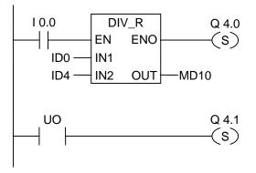
The box is activated by signal state "1" at I0.0. If the value of ID0 or ID4 is an invalid floating-point number, the math function is invalid. If the signal state of EN = 1 (activated) and if an error occurs during the processing of the function DIV\_R, the signal state of ENO = 0.
