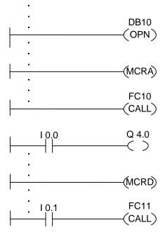
The Ladder rungs shown above are program sections from a function block written by a user. In this FB, DB10 is opened and MCR functionality is activated. If the unconditional call of FC10 is executed, the following occurs:
