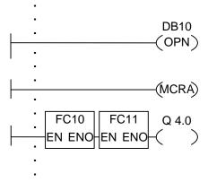
The Ladder rungs shown above are program sections from a function block written by a user. In this FB, DB10 is opened and MCR functionality is activated. If the unconditional call of FC10 is executed, the following occurs:
