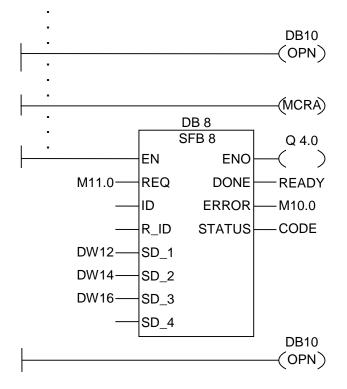
The Ladder rungs shown above are program sections from a function block written by a user. In this FB, DB10 is opened and MCR functionality is activated. If the unconditional call of SFB8 is executed, the following occurs:
