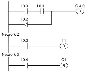
The signal state of output Q4.0 is reset to "0" if one of the following conditions exists:
