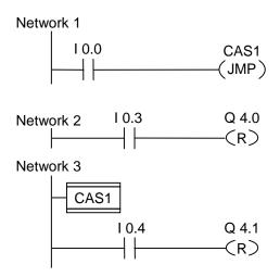
If 10.0 = "0", the jump to label CAS1 is executed. Because of the jump, the instruction to reset output Q4.0 is not executed even if there is a logic "1" at 10.3.
