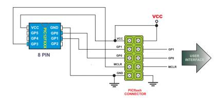
Connection schematics for 8 pin 12F PIC Microcontrollers. Some of the examples of 12F family are: PIC12F508, 509, 629, 635, 675, 683...
