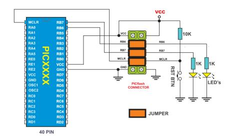
Once the development of a device is finished the jumpers have to be restored for enabling the device to work without PICflash programmer.
