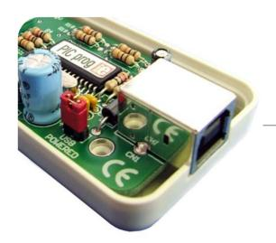
This picture shows the position of jumper when the target board and *PICflash* programmer are powered trough USB connector.
