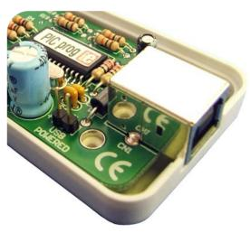
This picture shows the position of jumper when *PICflash* programmer is powered by the target board (target board have its own power supply).
