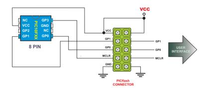
Connection schematics for 8 pin 10F PIC Microcontrollers. Some of the examples of 10F family are: PIC10F200, 2002, 2004, 206...
