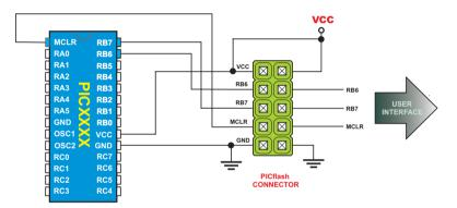
Connection schematics for 28 pin 16F and 18F PIC Microcontrollers. Some of the examples are: PIC16F876, 73... PIC18F252, 248, 2330...
