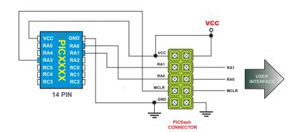
Connection schematics for 14 pin 16F PIC Microcontrollers. Some of the examples are: PIC16F676, 684, 688... USB In System Programmer for Microchip PIC microcontrollers
