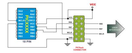
Connection schematics for 18 pin 16F and 18F PIC Microcontrollers. Some of the examples are: PIC16F84A, 88, 628, 716.... PIC18F1220,1320 ...
